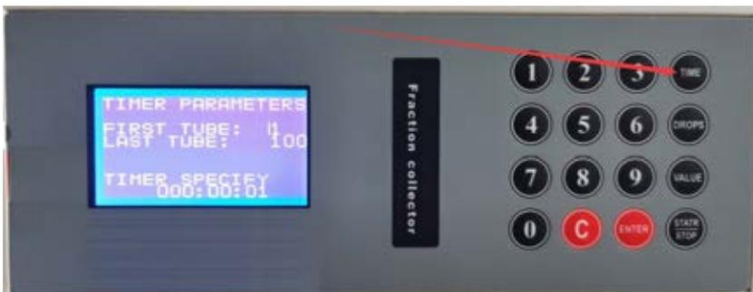
Set the parameter of "FIRST TUBE" to "1" and press "ENTER";
