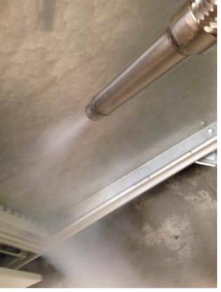
Open the enclosure door and locate the liquid nitrogen isolation valve. Using gloves and eye protection slowly open the valve while holding the dispensing hose.
