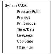
Pressure point: adjust the atmosphere value according to local atmosphere. The boiling point will be automatically calculated according to the atmosphere value.
