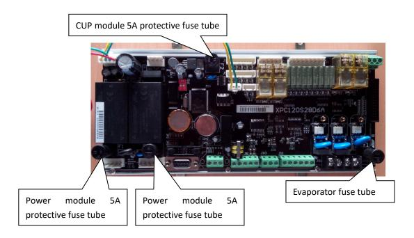
There are corresponding fuse in the equipment accessories, if there is a fuse burn out, find corresponding specification of fuse to replace it.
