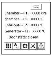
Chamber-P1: Indicates the chamber pressure
