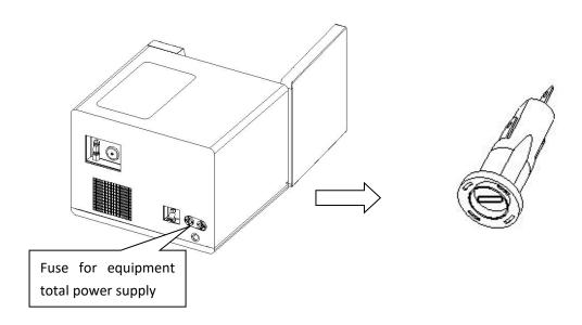
Firstly cut off the power supply connected to the equipment.
