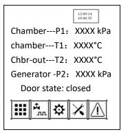
Chamber-P1: Indicates the chamber pressure
