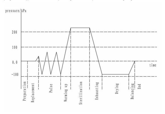
Instruction: When the product is not equipped with the vacuum function, the process is the positive pressure pulse
