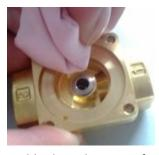
Clean up the sealing surface and re-install the solenoid valve.
