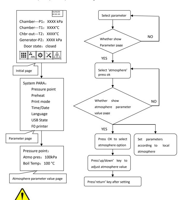
Adjust the atmospheric pressure value according to the local atmospheric pressure and the boiling temperature will be calculated automatically.
