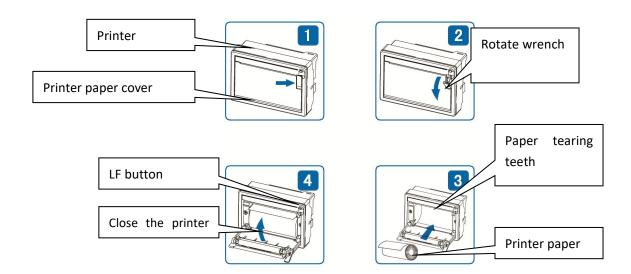
**NOTICE** When you see the red print on the printing paper roll, please replace the roll with a new one. Unsheathe the circumrotated wrench from the position the arrow point to as shown in Fig.1 and circum-gyrate it until the paper cover opened as shown in Fig 2.
