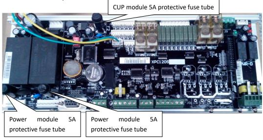
There are corresponding fuse in the equipment accessories, if there is a fuse burn out, find corresponding specification of fuse to replace it.
